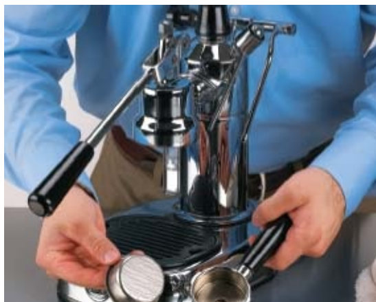
Manual piston machine. In the piston's long handle, pressure builds up until you release it
